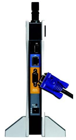
Figure 4-1: Monitor/Projector Connection
